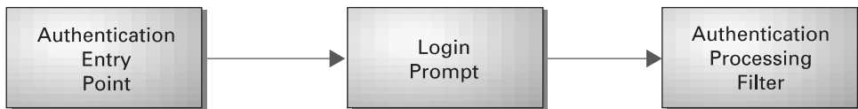
Figure 11.8 Authentication entry points and authentication-processing filters work together to authenticate a web user.
